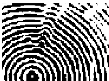
Fig. 1. Binarized image of a reflected Placido ring pattern taken by an existing corneal topographer. The skipped and uncorrected ring-points form a wedge-shaped artifact in the ring-pattern. Its effect on the optical power map is shown in Fig. 2
