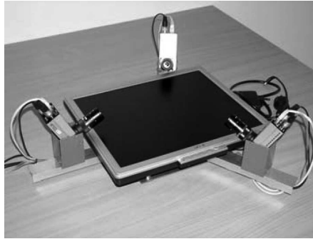
Fig. 4. The camera system of the multi-camera corneal topographer arrangement.
