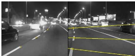
Fig. 1. Stereo matching: the correspondent of the highlighted points in the left image is searched along epipolar lines in the right image.
